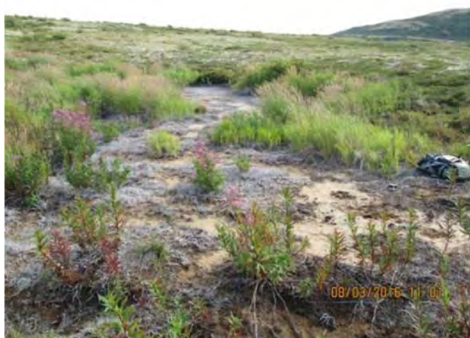
Figure 3: Dead vegetation and acidic drill cuttings (light-colored material in foreground) remain years after the hole was drilled. Soil was over 100 times higher in copper and molybdenum than background. The nearest hole (DDH 6355) was drilled in 2006.
