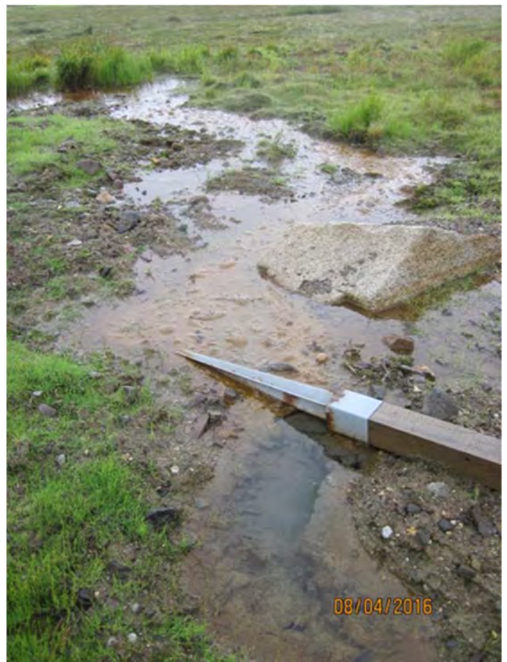
Figure 2: Artesian flow at DDH 9475, drilled in 2009.
