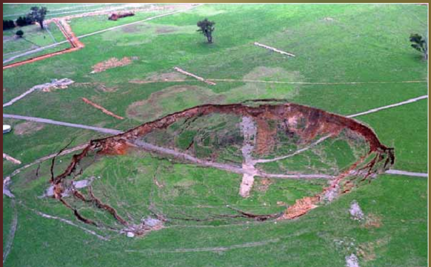
Figure 4. Subsidence due to block caving at the Ridgeway Mine, New South Wales from Newcrest Ltd. Cadia Operations, available at http://en.wikipedia.org/wiki/Image:Elura.png#file
