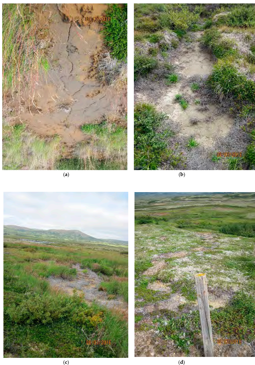
Figure 4. Oxidized and unoxidized cuttings from drill waste. Drill waste has a very fine texture and presents as either a gray color (unoxidized cuttings) or yellow–orange (oxidized cuttings). Drill waste was disposed of on land possibly 10–12 years prior to when these photos were taken in August 2016. (a) The fine texture and a mix of oxidized and unoxidized material, from widespread disposal near site DDH 6355, (b) Unoxidized cuttings, near site DDH 4145, (c) Swath of dead vegetation near DDH 6355, (d) Trail of drill cuttings from drill stem at DDH 4232. Photo credit: K. Zamzow.
