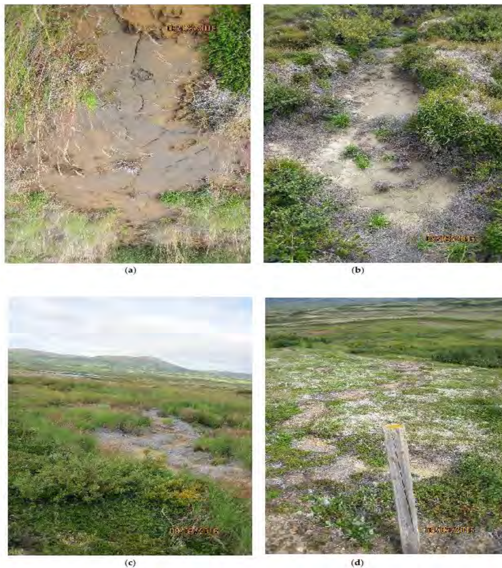
Fig. 4. Oxidized and unoxidized cuttings from drill waste. Drill waste has a very fine texture and presents as either a gray color (unoxidized cuttings) or yellow–orange (oxidized cuttings). Drill waste was disposed of on land possibly 10–12 years prior to when these photos were taken in August 2016. (a) The fine texture and a mix of oxidized and unoxidized material, from widespread disposal near site DDH 6355, (b) Unoxidized cuttings, near site DDH 4145, (c) Swath of dead vegetation near DDH 6355, (d) Trail of drill cuttings from drill stem at DDH 4232
