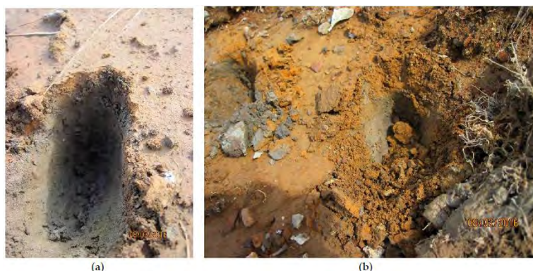
Fig. 6. Drill waste samples. (a) Site DDH 6355. The upper oxidized layer, with a field pH of 2.9, was submitted for analysis. A mixture of upper and lower layers had a field pH of 5.3. (b) Site DDH 5326. The upper and lower layers when mixed had a field pH of 6.4; the sample was not submitted for analysis
